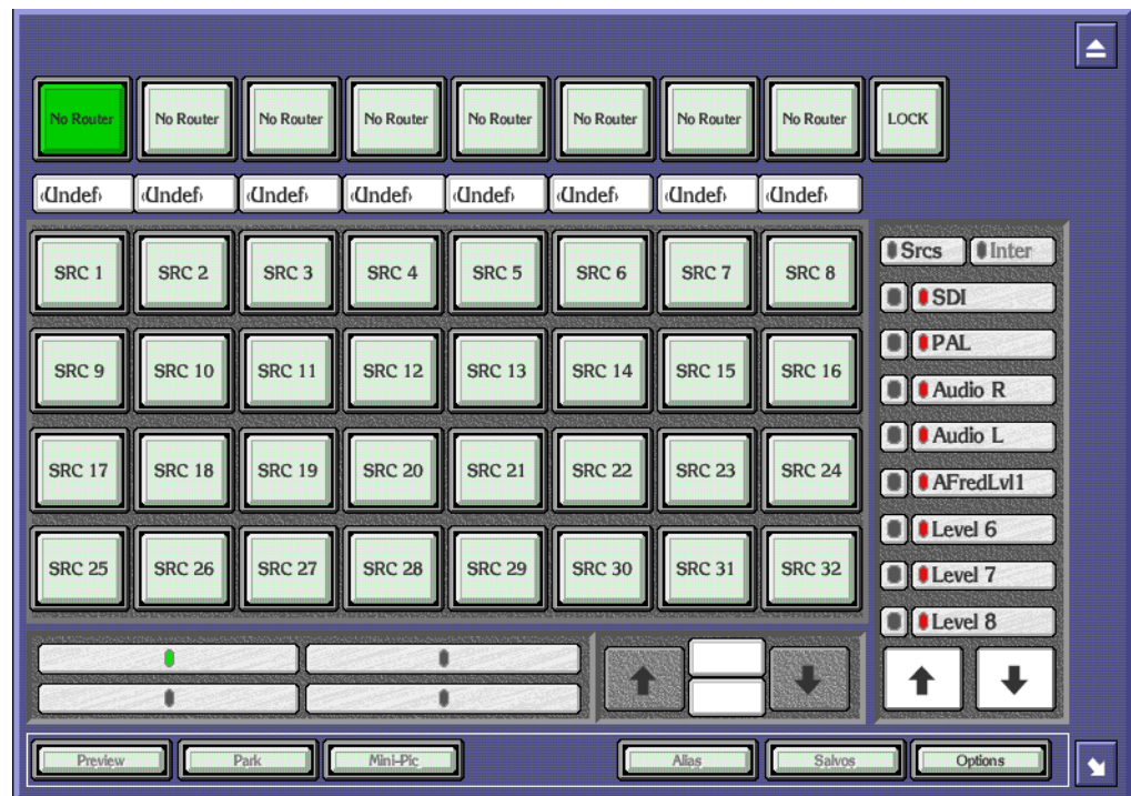
Figure 90. Typical Local Router Panel - Main Screen
