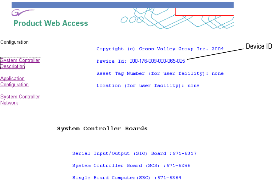
Figure 46. System Controller Description Window
